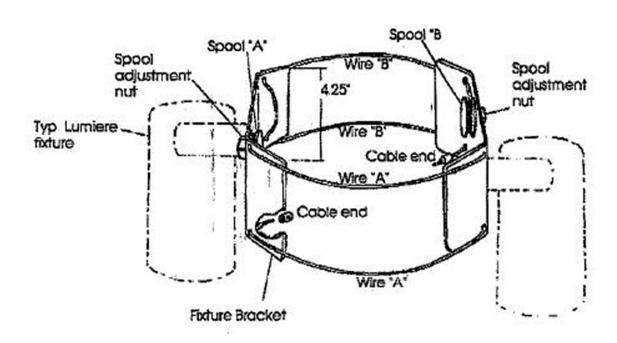
DESCRIPTION: Self adjusting tree strap designed to expand in diameter as the tree grows to prevent damage or restriction to the tree. Stainless steel cable connect 1 to 4 mounting brackets which hold standard accent fixtures. Cables are terminated on a tension controlled spool which slowly releases as the tree grows.
