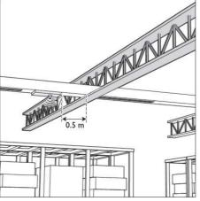
Do not install the InterAct System control unit close to steel or concrete constructions.
