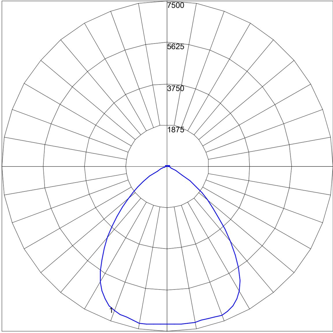
Maximum Candela = 7234.5 Located At Horizontal Angle = 175, Vertical Angle = 10
