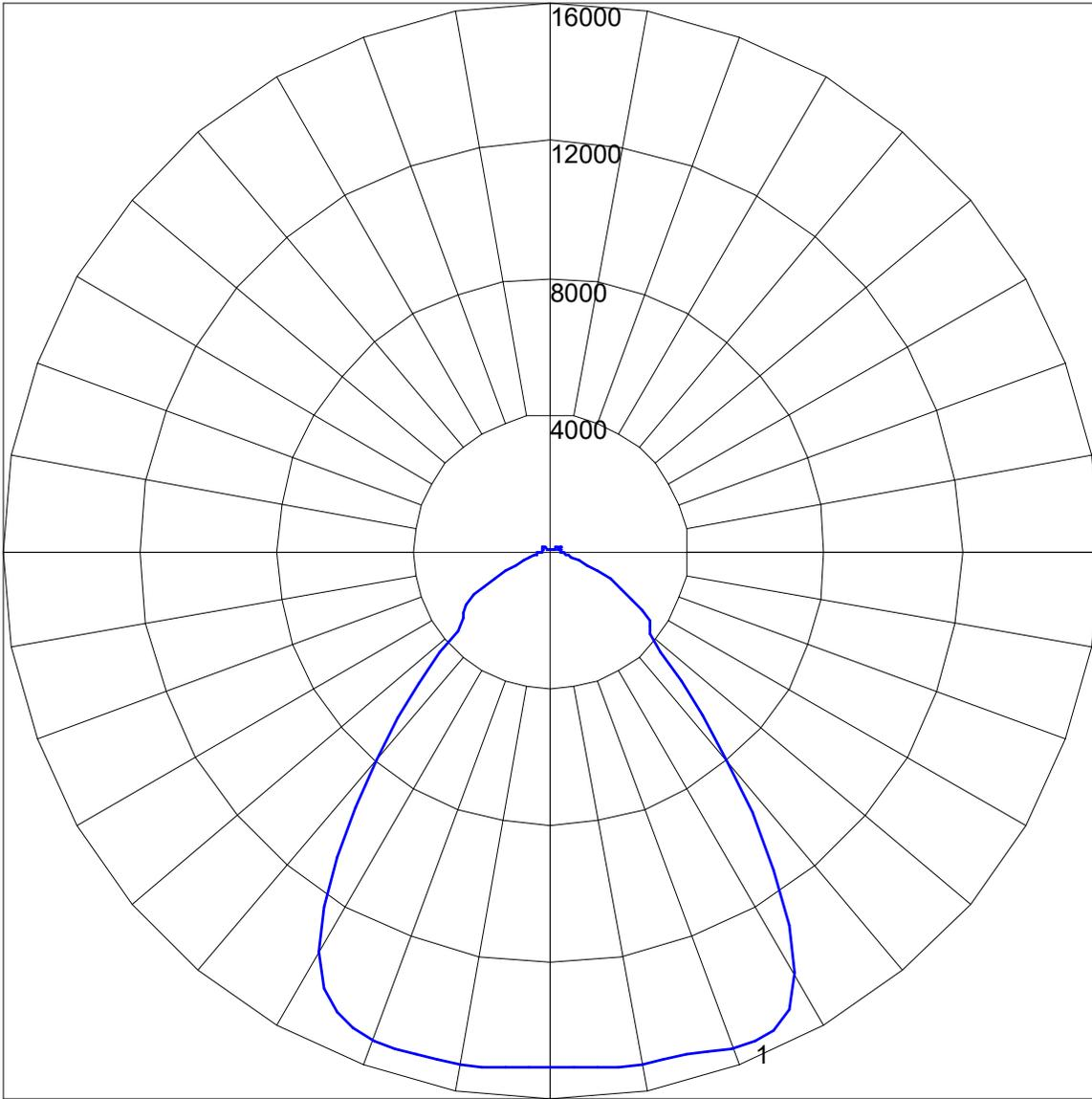
Maximum Candela = 15495.1 Located At Horizontal Angle = 0, Vertical Angle = 22.5
