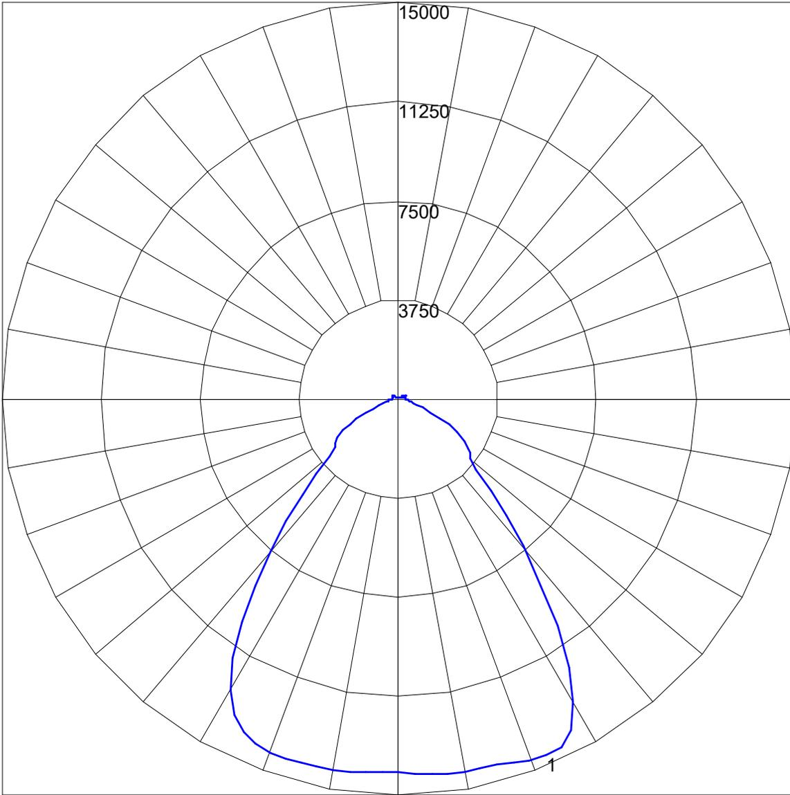
Maximum Candela = 14590.6 Located At Horizontal Angle = 0, Vertical Angle = 22.5
