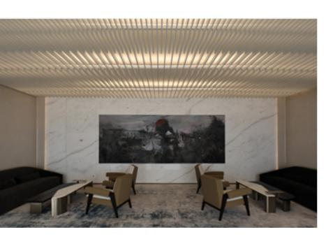
In addition, the healthy lighting concept of the WELL Building Standard has been well-addressed in this project. The lighting design largely applies light diffusion techniques and innovatively leverages indirect linear strips installed on the ceiling to aid diffuse lighting and offer larger expanses of continuous and ideal illumination. This results in improved aesthetics and occupant comfort, and ultimately creates a smart, green, and healthy building for CFC.
