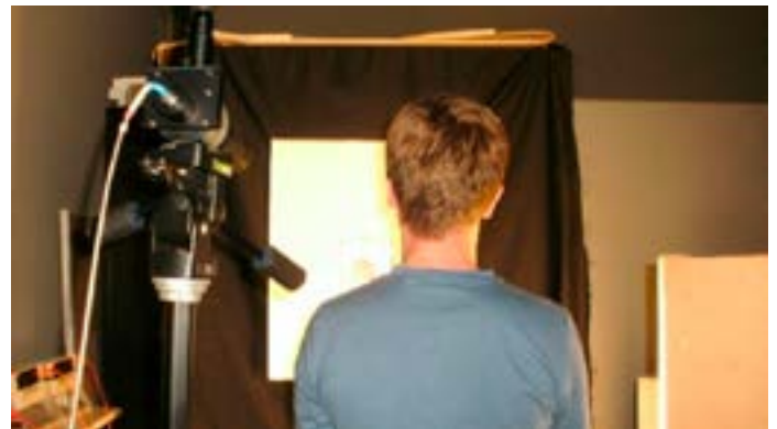
Figure 1: Test set-up with a telescope linked to a spectrophotometer on the left, and on the right a light box which test subjects must look into to erase the color from their retinas.
