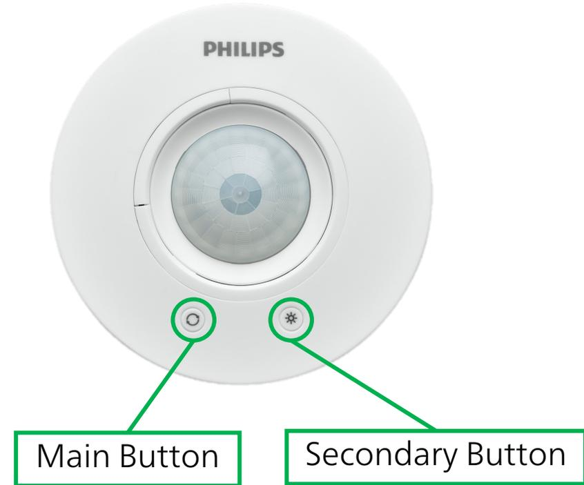
Two functional buttons exist on the front face: the left one is main button is used for grouping. The secondary button on the right is used to enable/disable sensing functions. An LED indicator is integrated for feedback and a retractable shield to reduce the motion detection field.
