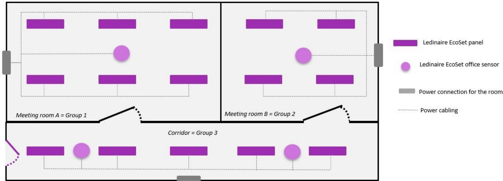
Figure 1 - Ensure powering for each group is independent
