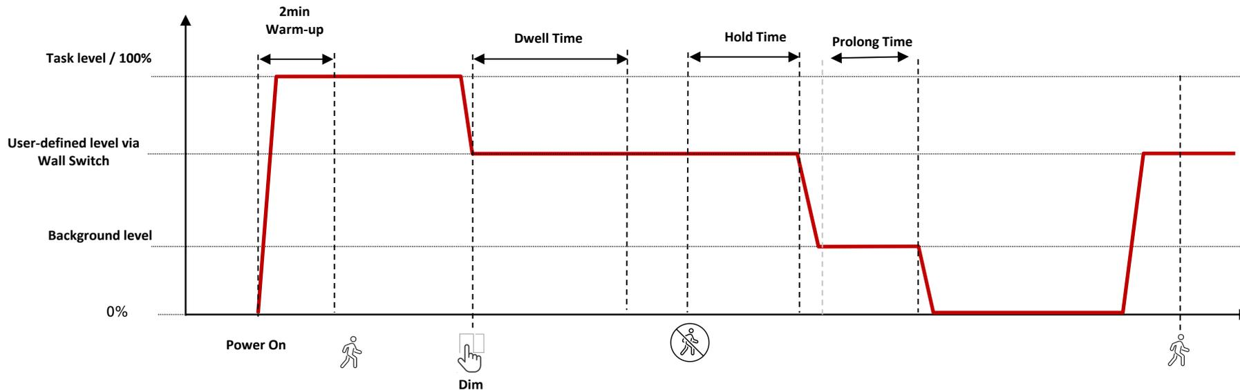
If a wall switch is used to change/dim the task light level, the system will keep the adjusted light level for an additional 30 minutes (dwell time), then the system returns to auto sensing control.
