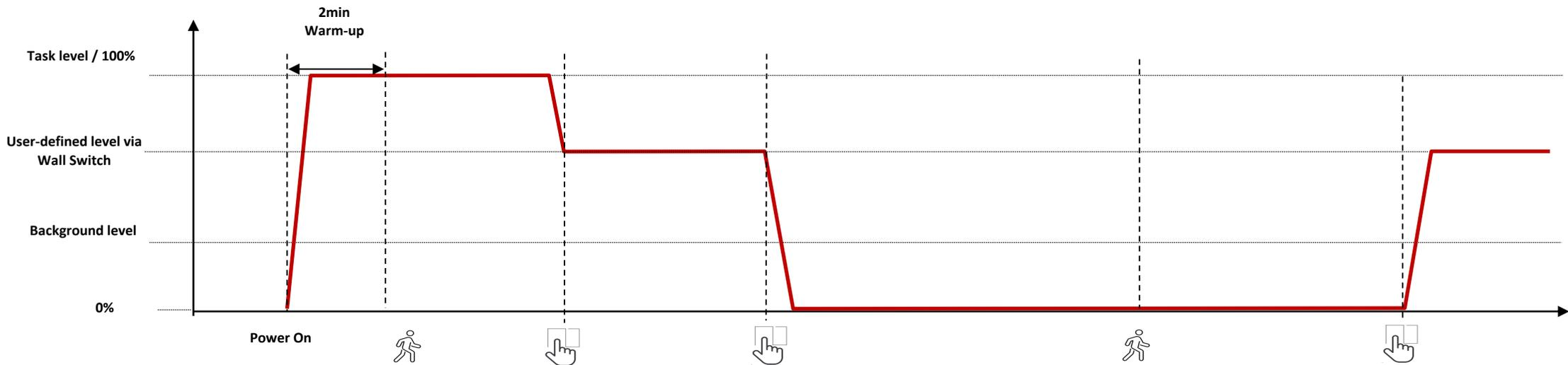
Where a group of luminaires have been manually switched to an off state with the EcoSet Wall switch, they will not react to motion detection in this state.
