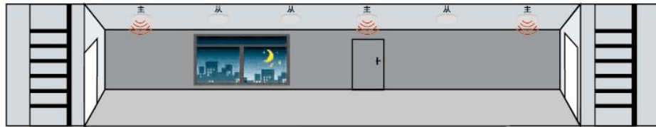
1 If no motion is detected, all lamps will be switched off.
