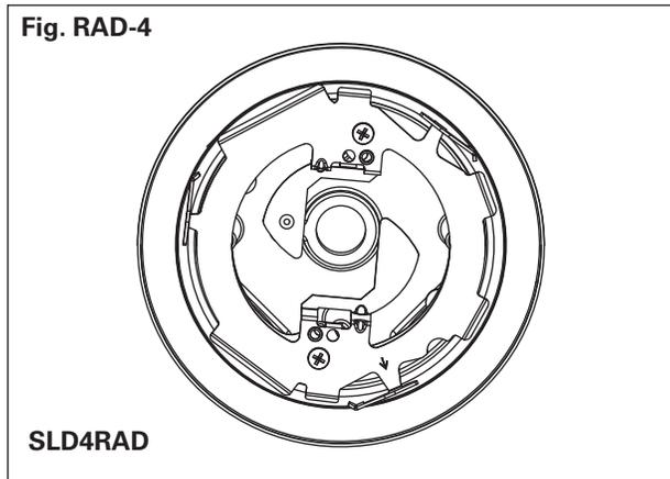
**SLDxRAD installation onto non-wet location junction box**
