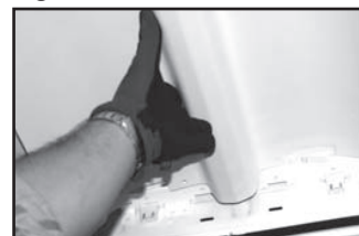
Figure 6. Reflector Slides into Lances
