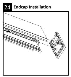
Slide endcap onto end of fixture module and secure from below using two #8-32 x 3/8" screws. Use ratchet to tighten screws until endcap seam is tight.
