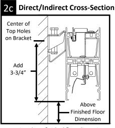
Determine above finished floor dimension and add 3-3/4" (96mm) for direct/indirect configuration. Draw center line through top holes on bracket, level and center wall brackets. Install to structure using appropriate hardware (by others).
