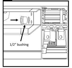
Determine power feed location on fixture. Attach supplied  $\frac{1}{2}$  bushing as shown.
