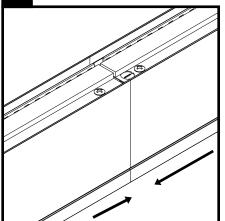
Ensure all connections are secure and all wires are fully tucked inside fixture wiring cavity. Slide fixture modules together gently. Level fixtures.
