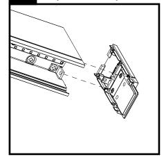
Place drop lens endcap as shown over the emboss of endcap and proceed with endcap Installation of endcap, step 31.
