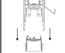
Remove one louver from end of fixture by pulling gently and temporarily suspend from available holes.
