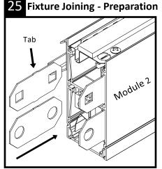
With module 2 on the ground, tap joiner aligners inside top and bottom screw chases as shown.
