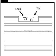
After module 1 is installed, adjust the tilt screw as required on each wall bracket to level fixture.
