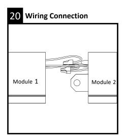
Bring modules close together, support module 2, complete wiring connections and tuck wires inside fixture wiring cavity. Engage joiner aligners from module 2 inside module 1.
