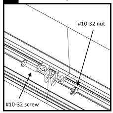
Secure fixture modules together using the two #10-32 machine screws and the two Self-locking #10-32 nuts supplied. Tighten until joint seam is tight.
