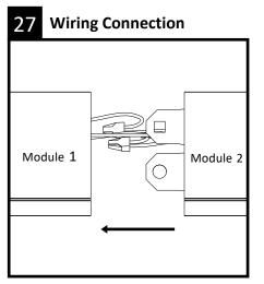
Bring modules close together, support module 2, complete wiring connections and tuck wires inside fixture wiring cavity. Engage joiner aligners from module 2 inside module 1.
