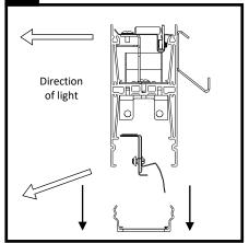
Remove lens and set aside until fixture installation is complete. Use cotton gloves to handle lenses and keep in a clean environment.
