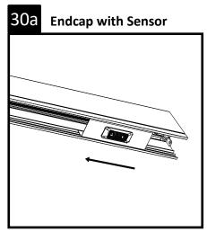
Before installing the endcap, slide the sensor towards the center of the fixture to gain access. Proceed with endcap installation, step 31.
