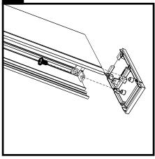
Slide endcap onto end of fixture module and secure from below using two #8-32 X 3/8" screws. Use ratchet to tighten screws until endcap seam is tight.
