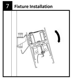
Hook fixture housing on top of wall bracket and gently rotate downwards while supporting housing. Housing should engage on all wall brackets and lock in position.
