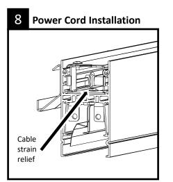
Feed power cord through ½" bushing installed in step 5. Crimp supplied cable strain relief to secure power cord inside fixture housing. Use a Heyco PN0019(R12) crimping tool to ensure proper installation.
