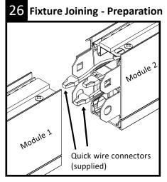
Raise module 2 to installed module 1 position. **IMPORTANT WIRING INSTRUCTIONS:** Quick wire connectors (supplied) are used for through wiring connections between fixtures. Wire nuts (by others) are used for connection of power junction box wiring to fixture wiring.
