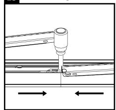
Ensure all connections are secure and all wires are fully tucked inside fixture wiring cavity. Slide fixture modules together gently. Insert 5/16" nut driver through 1/2" hole in top of reflector and tighten screw. Check that joint seam is tight. NOTE: Remove light engine pan before tightening joint.
