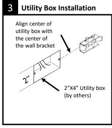
Determine power location for 2"X4" utility box (by others). Prior to installation, ensure center of utility box is centered on wall bracket center line as shown. Recommended position of utility box is 6" to 8" away from fixture end. See diagram on
