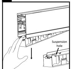
DO NOT ALLOW LOUVER TO HANG FROM ELECTRICAL WIRES.
