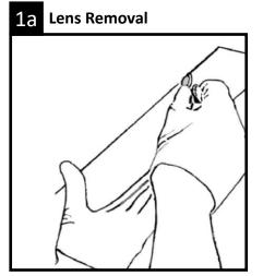
Lens Removal: To remove snap-in lens for maintenance purposes, insert a flat, smooth edged object between lens and housing (avoid screwdrivers). Twist to release pressure and remove lens.
