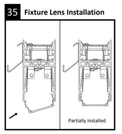
Install lenses removed in step 1.
