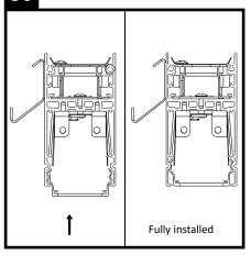
Once lens is positioned inside housing, starting on one end or joint, push upwards gently and work outward to complete the run.
