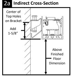
Determine above finished floor dimension and add 1-5/8" (42mm) for indirect configuration. Draw center line through top holes on bracket, level and center wall brackets. Install to structure using appropriate hardware (by others).
