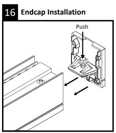
**NOTE:** Remove light engine pan before installing endcap. Slide endcap towards fixture bracket until it engages and clicks in place. Push down on bolt to help engage if needed.
