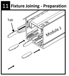
With module 2 on the ground, tap joiner aligners inside top and bottom screw chases as shown. To allow for proper joining, ensure aligner tab in the middle is fully inserted inside module 2 housing, approximately 1/4" past the middle point.
