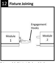
Raise module 2 to installed module 1 position.
