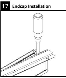
Insert 5/16" nut driver and tighten screw until endcap seam is tight. **NOTE: Do not overtighten.** Reinstall light engine.
