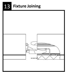
Bring modules together and engage joiner bracket in module 1 on fixture bracket in module 2. Ensure slots on module 2 fixture bracket lock on hooks of module 1 joiner bracket.
