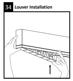
Installation Tip: For easier installation, start on one end of the louver pressing gently on side tabs. IMPORTANT: For asymmetric louver fixtures, orient the arrows on the louver pan to point at the label on the outside of the housing.
