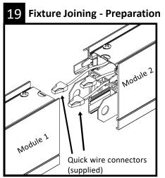
Raise module 2 to installed module 1 position. **IMPORTANT WIRING INSTRUCTIONS:** Quick wire connectors (supplied) are used for through wiring connections between fixtures. Wire nuts (by others) are used for connection of junction box wiring to fixture wiring.
