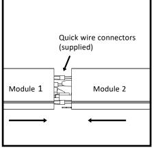
Bring modules close together, support module 2, complete wiring connections and tuck wires inside fixture wiring cavity. **IMPORTANT WIRING INSTRUCTIONS:** Quick wire connectors (supplied) are used for through wiring connections between fixtures. Wire nuts (by others) are used for connection of power drops wiring to fixture wiring.
