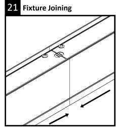
Ensure all connections are secure and all wires are fully tucked inside fixture wiring cavity. Slide fixture modules together gently. Level fixtures.
