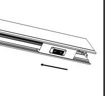
Before installing the endcap, slide the sensor towards the center of the fixture to gain access. Proceed with endcap installation, step 24.
