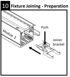
Slide joiner bracket into fixture bracket until it locks in position. Push down hex bolt and spring on joiner bracket to engage with internal bracket.
