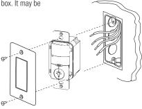
CAUTION: Before installing or performing any service on a Greengate system, the power MUST be turned OFF at the branch circuit breaker. According to NEC 240-83(d), if the branch circuit breaker is used as the main switch for a fluorescent lighting circuit, the circuit breaker should be marked "SWD." All installations should be in compliance with the National Electric Code and all state and local codes.
