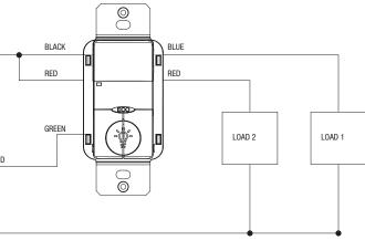
Wiring Diagram 2: 120/277 VAC dual level dual circuit wiring diagram
