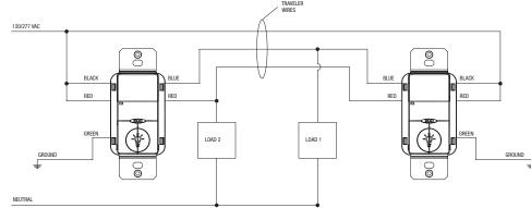
THREE-WAY WIRING DIAGRAM
