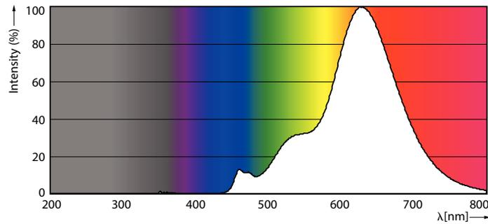
Spectral Power Distribution Colour - CLA LEDBulb D 5.5-25W ST64 E27 GOLD SP C
