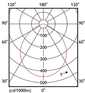
Light Distribution Diagram - DN060B LED8S/830 PSU WH
