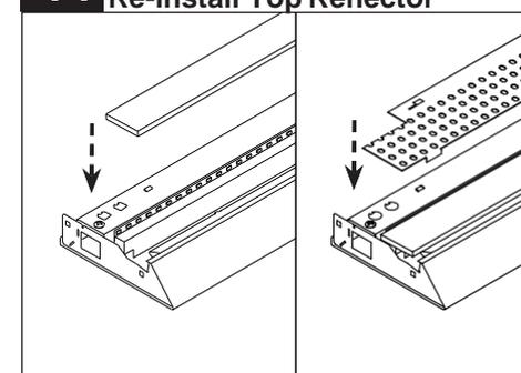
**Identify smooth side of the Light Guide and ensure it is installed smooth side DOWN.**
