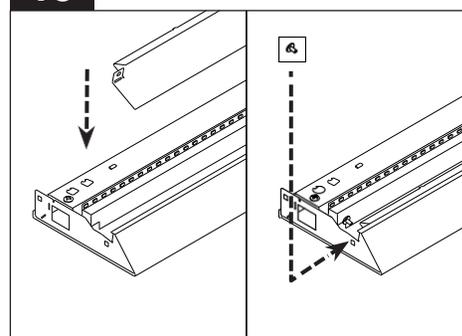
Re-install front reflector using short (stubby) screwdriver.
