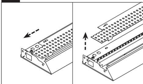
Shift top reflector to the left and then remove the reflector.
