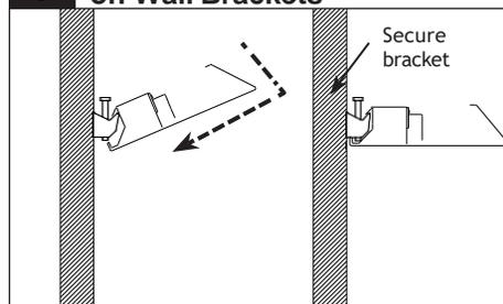
With 2 people, raise fixture into position and engage it on hooks located on top of wall brackets, then rotate it down into position. Secure bracket using supplied hardware.
