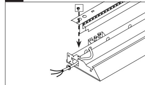
To access wiring, remove screw from top pan and lift pan off. Apply strain relief to power cord.
