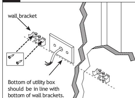
Determine fixture mounting location and secure wall brackets to structure using appropriate fasteners (two per bracket, supplied by others). 4ft fixtures: Require two bracket assemblies; 8ft fixtures: Require three bracket assemblies. Brackets must be installed a maximum of 5" from end of fixture (on 8ft fixture, the third bracket can be 5" of other side of inrow crossplate).
