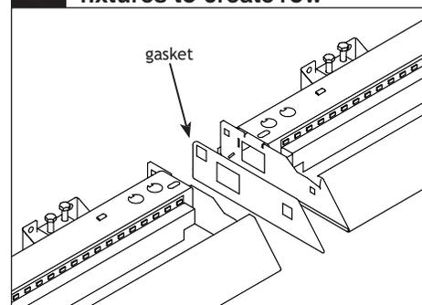
With two people, raise second fixture and engage on mounting brackets (see STEP 4). At joint, remember to insert black gasket.
