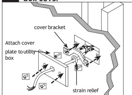
Determine power feed location and install 2"x4" utility box (supplied by others) parallel with fixture. Complete connections at utility box with supplied power cord. Attach cover bracket using supplied hardware. Punch power access hole in supplied cover, feed power cord through and attach strain relief on wall side. Attach cover using supplied painted hardware. NOTE: Bottom of utility box should be in line with bottom of wall brackets.
