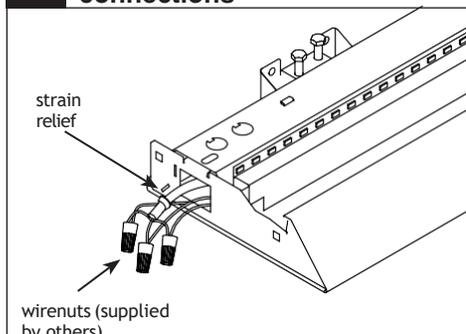
Complete electrical connections using wire nuts (supplied by others). Re-install pan and hardware removed in STEP 5.
