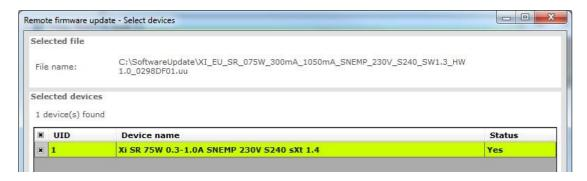
All supported devices for this update procedure are retrieved and listed. The status column describes the reason why a device is or isn't supported. The user can select the devices from the list and when one or more supported devices are selected the
