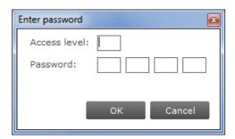
After providing a correct access level and password, and clicking **OK**, the OEM Readout-protected features will be read. By clicking **Cancel** none of the selected features will be read. If an incorrect access level and/or password were provided, the OEM Readout-protected features will receive a status icon indicating failure (see below).
