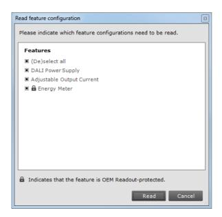
If an OEM Readout-protected feature is read, a dialog will appear asking for an access level and a password.
