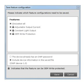
In this case it is possible to save the current password alongside the features, so MultiOne Workflow can use this password to be able to write the data of the features that are OEM Write-protected to the driver.
