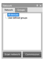
**Note!** A **Scan network** or **Commission** execution will place all found devices into manufacturer specific operating mode. Take care of this in case you need to use a connected driver in the DALI standard operating mode!
