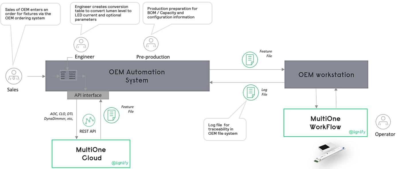
The figure above represents the process flow. The sales personnel/technician enters the sales order, and the details are then converted to driver specific information. Based on this information in the automation system, the system makes specific API calls to connect with MultiOne Cloud as described in this document. In this way the feature files can be generated automatically and can be used in the production for configuring drivers.
