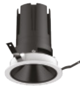
Ø115*64mm Hole Size \text{\textcircled{D}} 100mm (The ceiling thickness is required to be 5-25mm)
