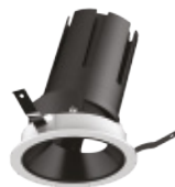
Ø115*64mm Hole Size \text{\textcircled{D}} 100mm (The ceiling thickness is required to be 5-25mm)
