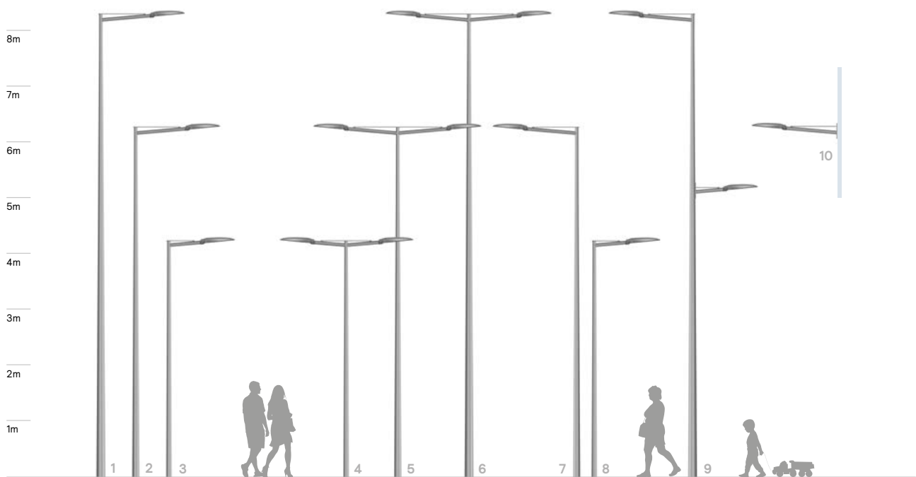
1-2-5-6-7. Modena LED gen2 + crosse Batio L1000 + mât Accante 3-4-8. Modena LED gen2 + crosse Batio L600 + mât Accante 9. Modena LED gen2 + crosse Batio L1000 + mât Accante + Modena LED gen2 + contre-feu Batio L600 10. Modena LED gen2 + applique murale Batio L1000
