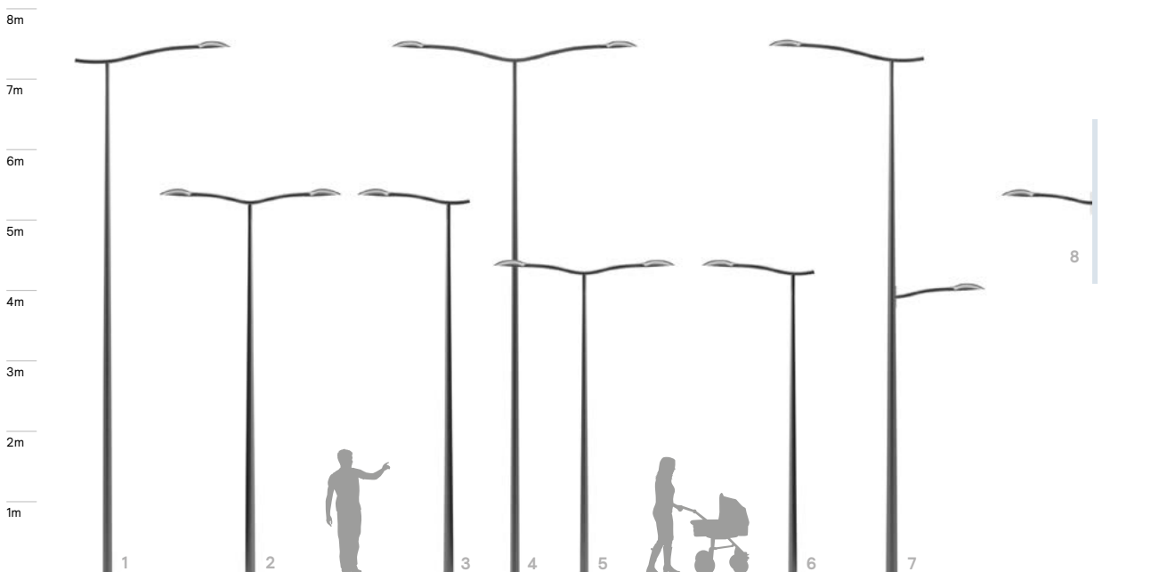
1-4. MileWide LED gen2 Large + crosse UrbanWave L1200 + mât Accante 2-3-5-6. MileWide LED gen2 Small + crosse UrbanWave L750 + mât Accante 7. MileWide LED gen2 Large + crosse UrbanWave L1200 + mât Accante + MileWide LED gen2 Small + contre-feu UrbanWave L750 8. MileWide LED gen2 Small + applique murale UrbanWave L750
