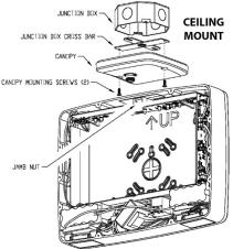
Ceiling Mounting –Mount junction box cross bar to junction box. Mount canopy to cross bar using screws provided in canopy kit. Place thin O-ring in the groove in the canopy around the canopy mounting stud. Remove left-most knockout in top of housing and secure exit housing to canopy mounting stud using jamb nut provided. Refer to Step 3 for wiring instructions.
