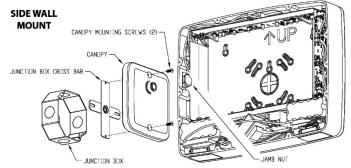
Side Wall Mount –Mount junction box cross bar to junction box. Mount canopy to cross bar using screws provided in canopy kit. Place thin O-ring in the groove in the canopy around the canopy mounting stud. Remove right-most knockout in top of housing and secure exit housing to canopy mounting stud using jamb nut provided. Refer to Step 3 for AC wiring instructions.
